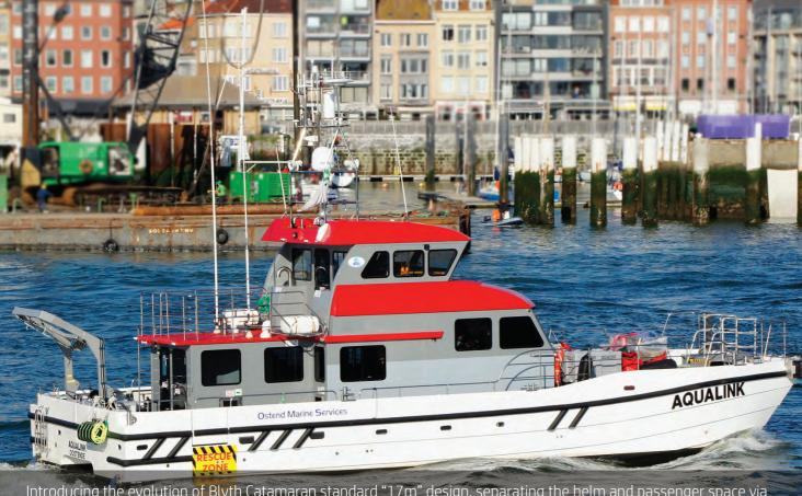
Introducing the evolution of Blyth Catamaran standard "17m" design, separating the helm and passenger space via the top wheelhouse. This ingenious layout allows for increased internal working space in the main cabin and can easily accommodate both survey and crew transfer duties.
